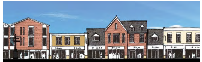
Fig 3.17: Above and below: A vertical rhythm and individual definition of each retail unit can be achieved in a range of architectural styles (image:© corstorphine+wright architects)
